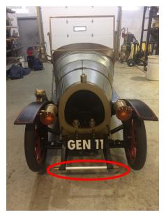
The **Crossbar located at the Front of the Prop** is the **Only load-bearing part forward of the dashboard**. It is intended to help lift the prop over bumps and as a tiedown point during shipping.
